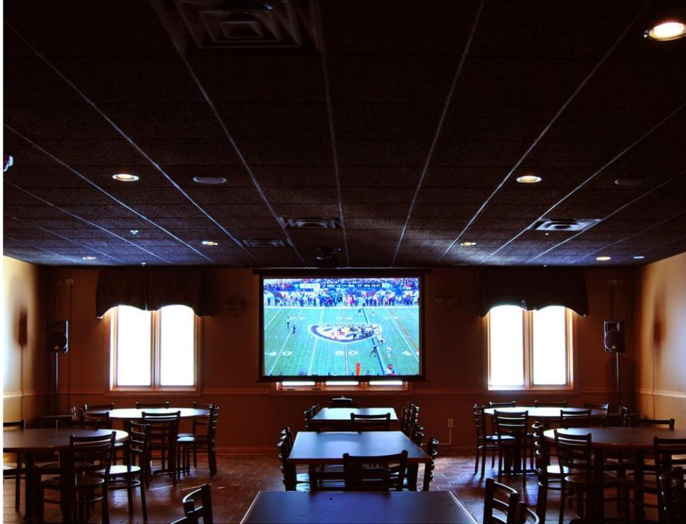
Also part of the installation were a private party room with a 106-inch screen with an HD projector and a 3,000-watt 5.1 surround stereo system, an audio system with two Niles SI-1230 amplifiers and an ELAN D12 amplifier to power 60 speakers, bringing hi-def audio and video to every guest in every seat in the house. The job also features fully integrated surveillance and security systems and plans to incorporate thermostats at the former Japanese steakhouse soon.
